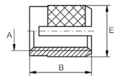
Female thread A = M2 Length B = 4.0Min distance to edge = 2.0Outer diameter E = 4.00
